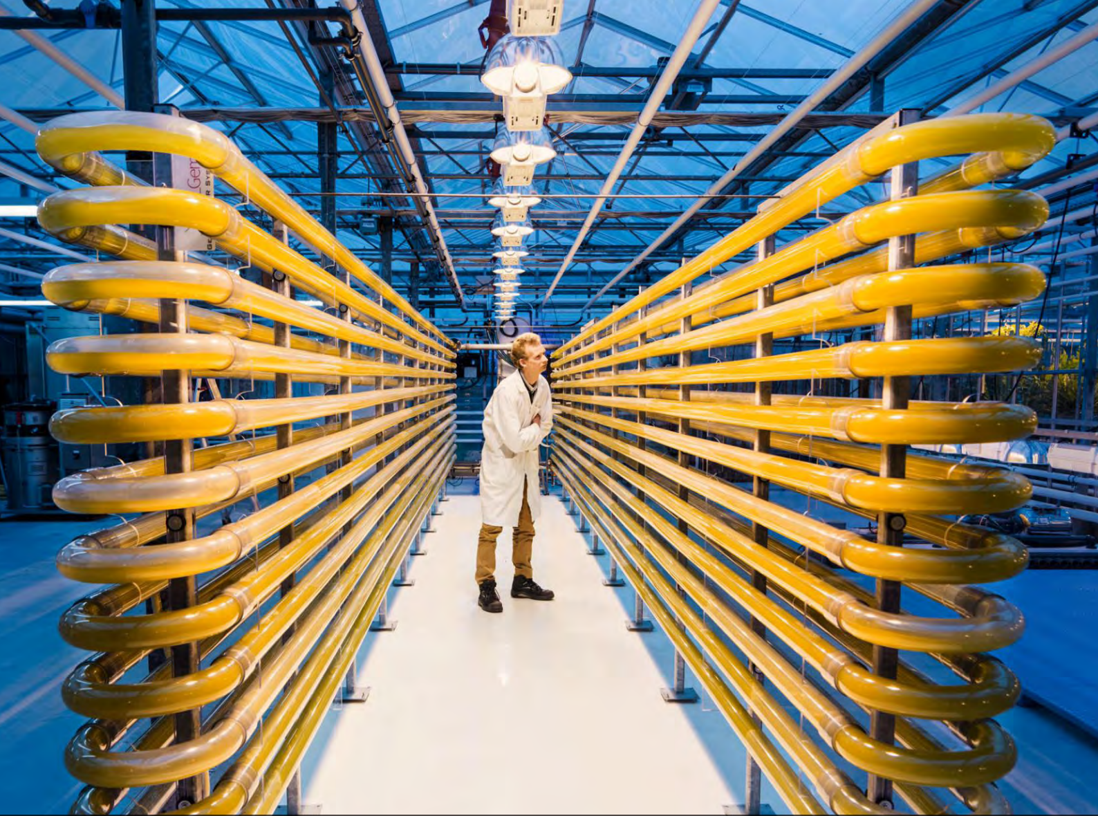
Ruud Veloo monitors an experimental “photobioreactor” at WUR’s AlgaePARC. Light fuels the growth of microalgae, which are used to produce proteins and lipids, the basis of many food chains.
